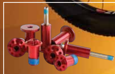
The Jet 9 is finished with custom machined and anodized pivot hardware.
